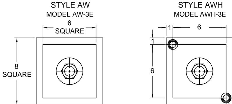
ELASTOMERIC GROMMET FOR 1/2 ANCHOR BOLTS (2 TYP)
